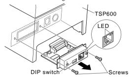
⑥ Once the interface board has been connected, perform a self-print test before connecting the Ethernet cable. Also, make sure that the printer recognizes the interface board. When recognized: Prints "Interface: NIC".
